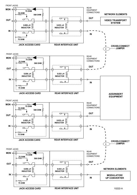
Figure 26. Cross-Connect Application for Local Commercial Insertion
